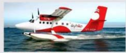
AMPHIBIOUS AIRCRAFT. SkyHop has secured a Twin Otter DHC-6-400 series aircraft, equipped with floats for water landing
