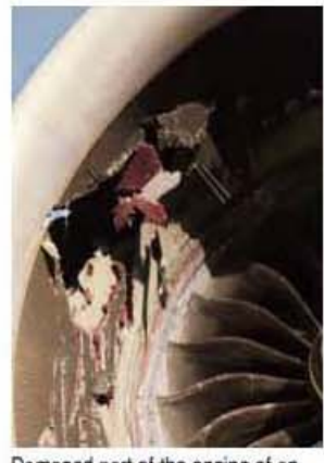
Damaged part of the engine of an Air India A350 aircraft PTI
