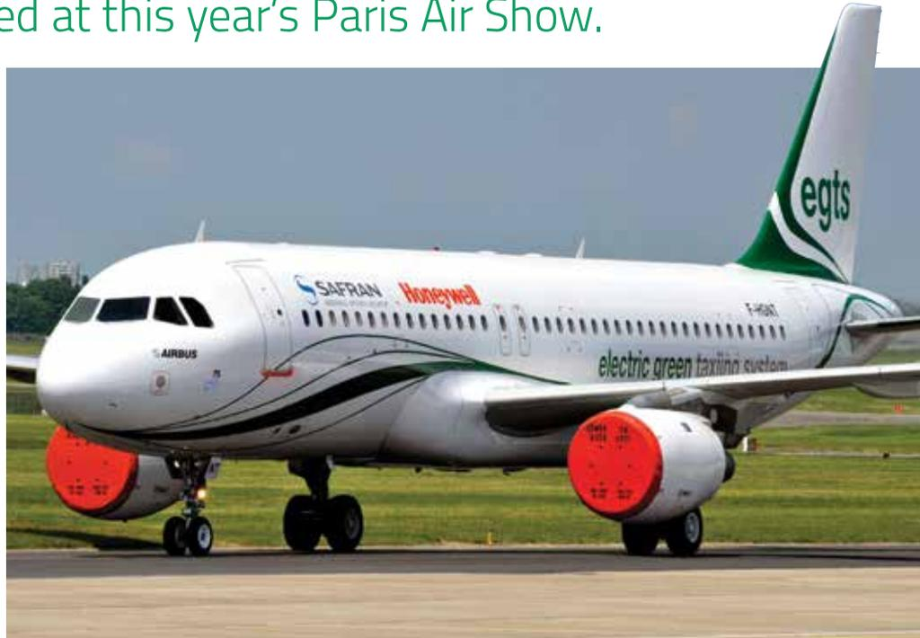
Engine covers on and no tow-tractor, but this A320 can still taxi thanks to its electrically-driven wheels. (EGTS)
