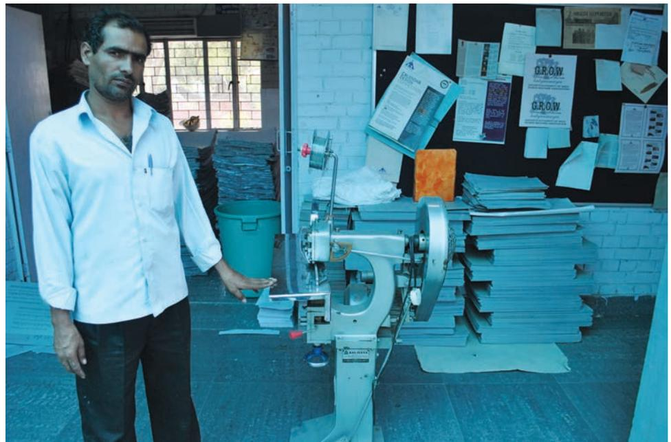
*Paper creasing and stitching machine at paper recycling unit of AAI*
